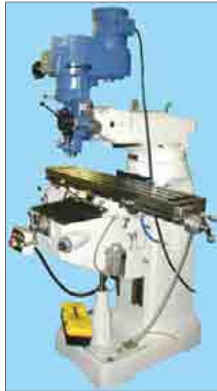
Variable speed knee-type milling machine.
