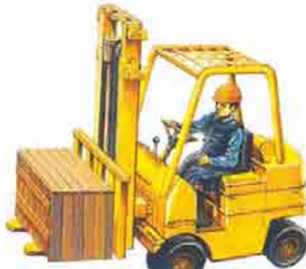
Fork lift is used to move goods from one place to the other within the factory.
