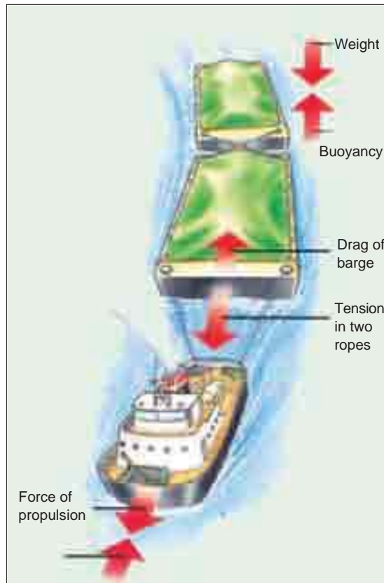
Forces on a ship as shown above need to be consider while designing various joints Note : This picture is given as additional information and is not a direct example of the current chapter.
